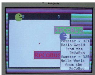
Fig. 8. Video output of the reconfigurable system. Each of the six objects (e.g., a text box) on the screen is created by an individual module. Each module receives the video stream from the I/O bar that is then overlaid with the particular object and sent further over the I/O bar to the next module.
