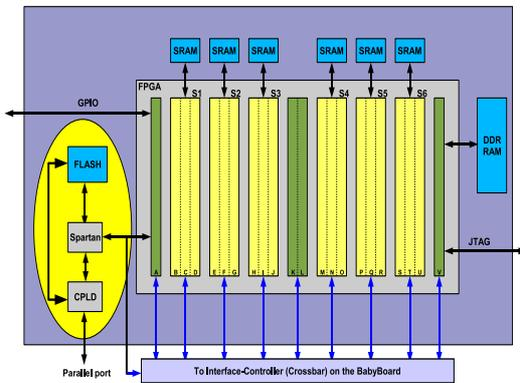
Figure 2. Architecture of the ESM-Baby board.
